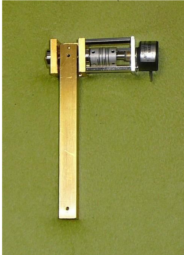
Fig. 8 Instead of locking with a nut, just putting an amount of silicone glue seems to be enough to keep this encoder in position.
