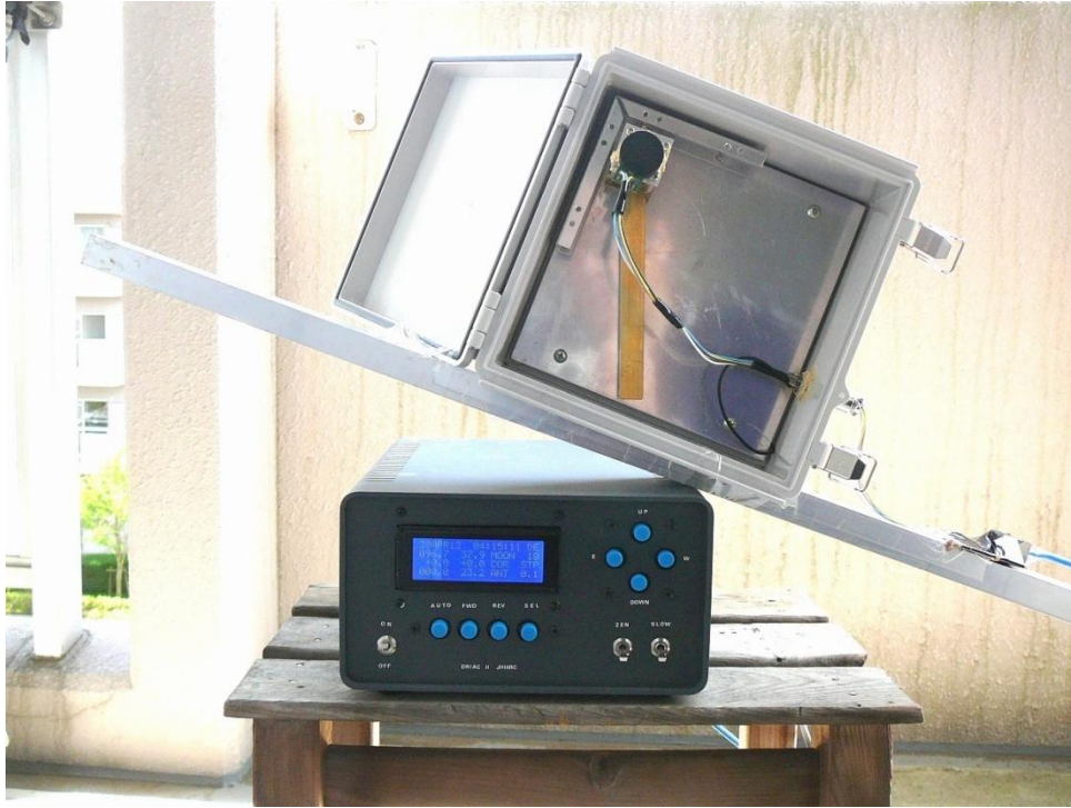
Fig. 10 Elevation angle detection was tested with an aluminum bar of 20x40x2000 mm long. A 35mm arc at the free end of the 2000mm bar makes 1 degree change in the elevation. This inclination was detected with the gravity-sensitive method.
