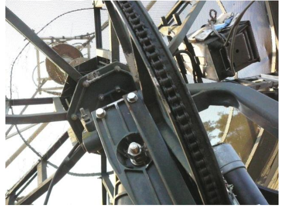
(Fig.1) 4.4m TVRO dish, a product of Paraclipse, at JH1KRC has no construction that fits for detecting the elevation angle directly at the elevation rotary axis.
